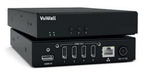
Plug and play with default output arrangement of 2x2 set for the most common scenarios. Output arrangement can be set from the front panel to additional simple arrangements: 2x1, 1x2, 2x2, 3x1, 1x3, 4x1, 1x4 in both portrait and landscape. Manage multiple AdScape units over the network with the AdScape Configurator software to customize output arrangements in mixed resolutions and bezel management.
